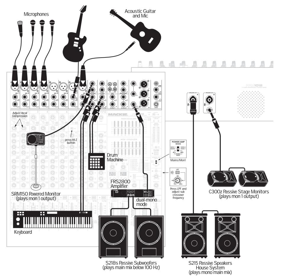
This diagram shows microphones attached to the mic inputs of channels 1 to 4, an electric guitar connected directly to channel 7 (with hi-z switch pressed in), an acoustic guitar microphone connected to channel 8 mic in, a keyboard attached to channels 9/10, and a drum machine to channels 11/12.
